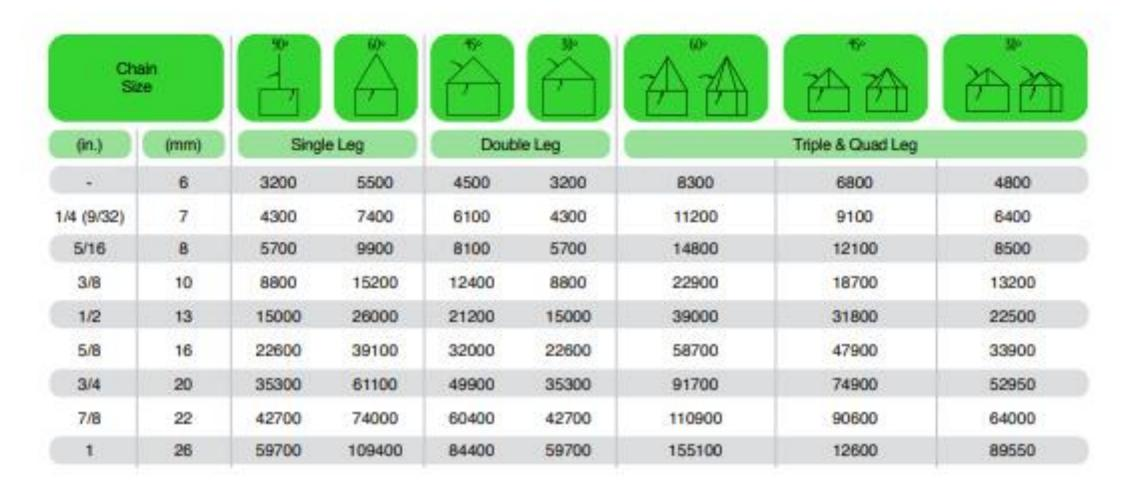
\*For choker applications, the working load limit must be reduced by 20%. The Crosby A-1338 cradle grab hook doesn't require any reduction of the working load limit. The design factor of 4:1 on Spectrum 10 alloy chain agrees with the design factor used by the International Standards Organization (ISO) and ANSI B30.9 and is the preferred set of working load limit values to be used.
